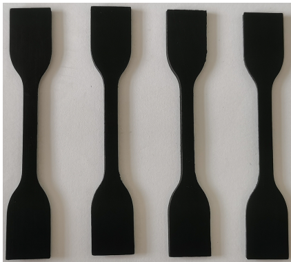
图 2 I 型哑铃形持久拉伸试样图 Fig. 2 Diagram of Type I dumbbell-shaped specimen for long-term tensile test
