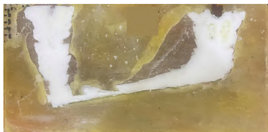
(c) 6号实验(管柱上提2次,垫层不提)
