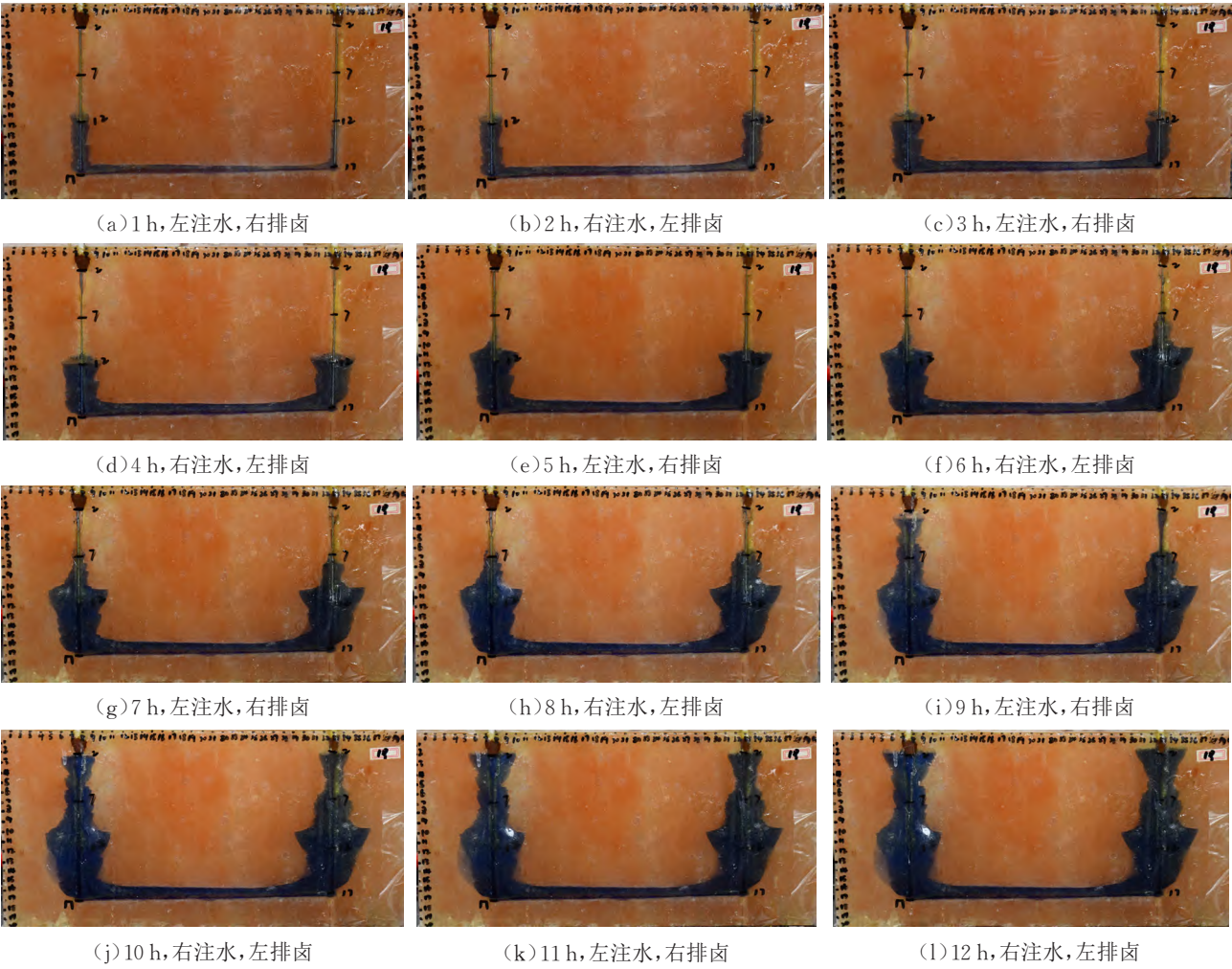
图 4 室内对接井水溶造腔腔体形态发展过程图 Fig. 4 Development process of docking well leaching using water solution in laboratory experiment
